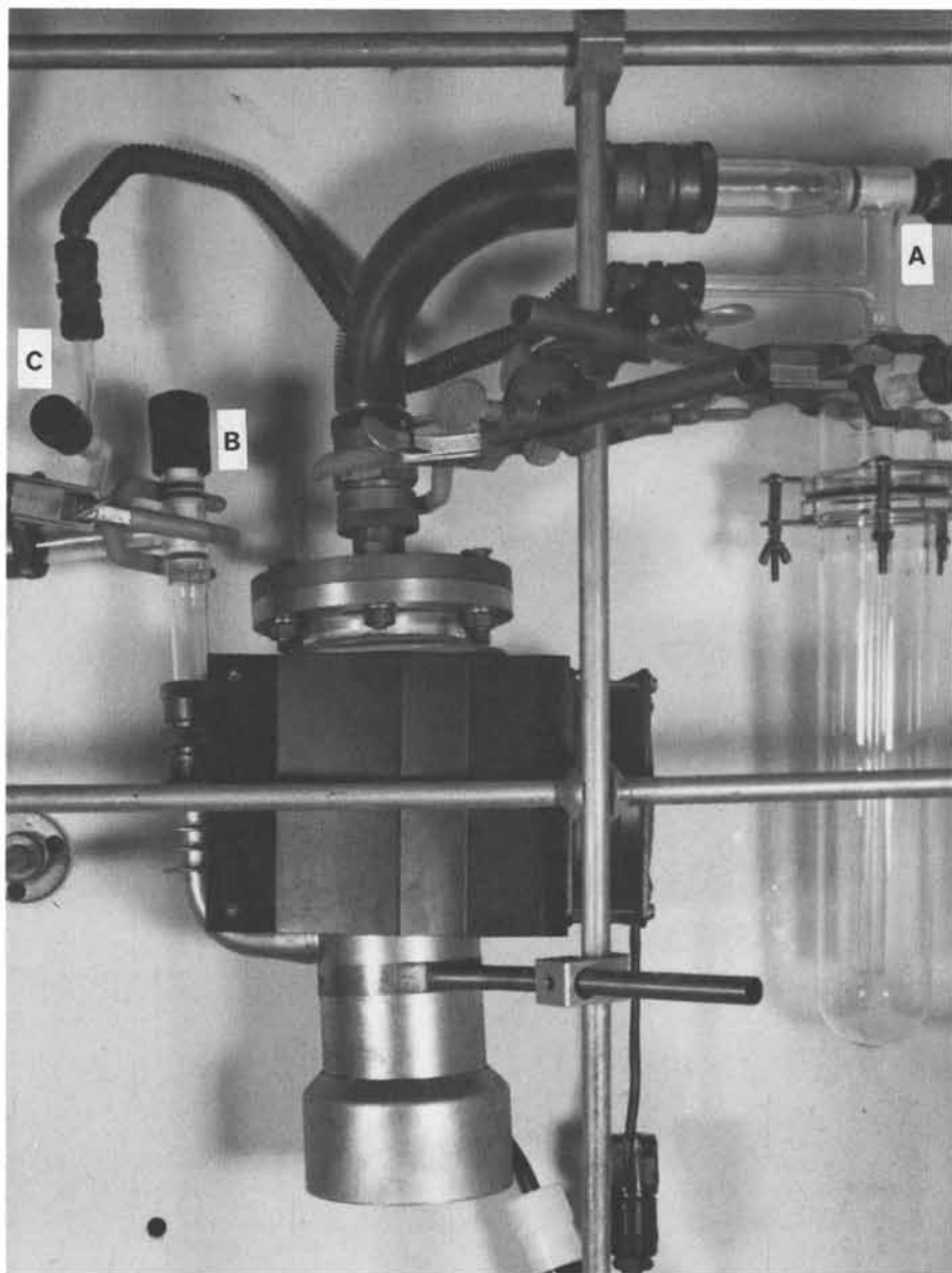
Figure 1. 3-Valve bypass design used on medium vacuum/Schlenk lines. Note position of valves labelled A, B and C. Also note 1.) the compact VEECO oil diffusion pump and 2.) the grease-free 57 mm O-ring flat-flanged trap used on this type of line.
