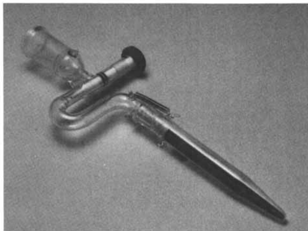
Figure 5. Graduated volume for addition of volatile liquids to reaction flasks.
